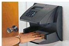
Figure 6. Hand Geometry Scanner.
