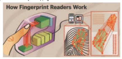
A few devices use newer silicon technology to record prints. In these *capacitive* units, esensors use the human body's natural electrical charge to measure the difference in potential energy between ridges and valleys in a fingerprint. This is also how they can tell whether the finger is "live."
