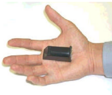
Fig. 8-1 The small size of the FDx01 optic sensor allows it to fit into all kinds of hand-held devices, including computer mouse and keyboard.
